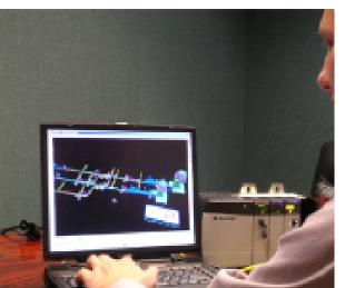
code. This is called a PolySim<sup>SM</sup> Emulation – the PLC reads the input from the model and directs the outputs to cause actions in the model, according to the logic.
