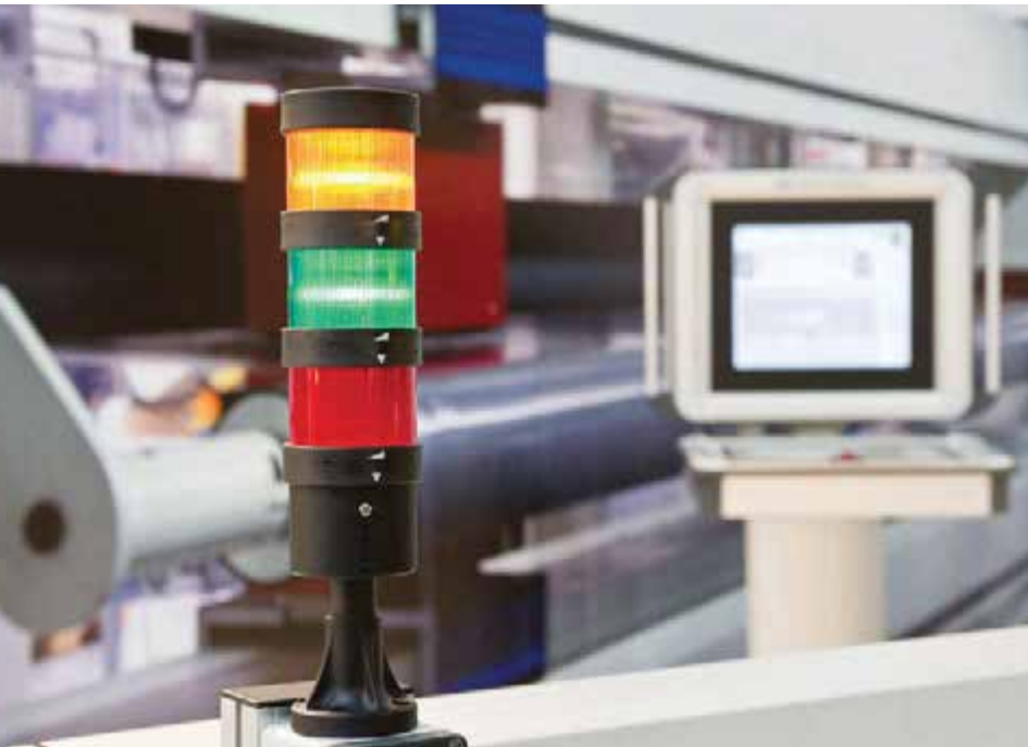
Updated human-machine interface (HMI) screens and safety alarm systems help improve operator and machine performance.
