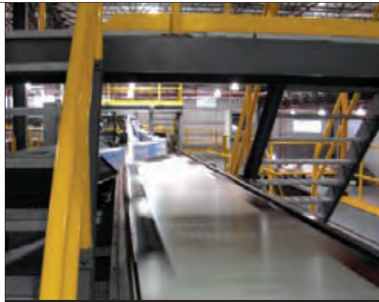
This sorter is diverting product into accumulation lanes.
