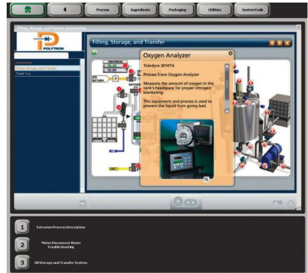
FIGURE 1: The future human-machine interface (HMI) can provide more real-time information for the user, allowing for smarter and better decisions. Images courtesy: Polytron
